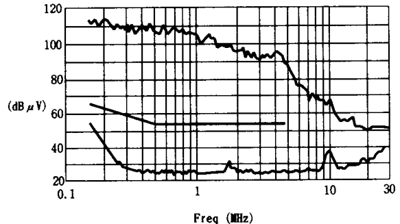
EU Standards EN55011 (Class B) measurement data
